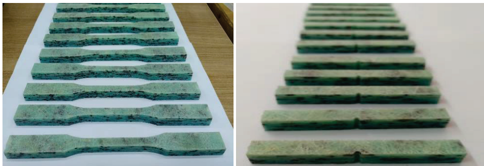
Fig. 7. Samples prepared for the static tensile test on the Zwick Roell machine made of EPO 5 material (a); Sample made of EPO 5 material prepared for impact tests on the Charpy RKP450 - TestXpert II pendulum hammer (b)
