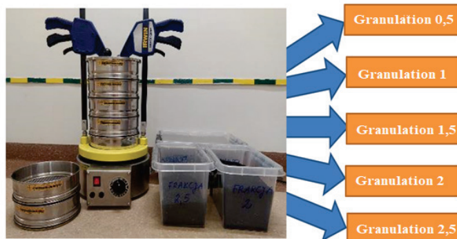
Fig. 5. Obtaining specific fractions of rubber recyclate with the use of a sieve shaker EKOLAB, model: LAB-11 -200/UP
