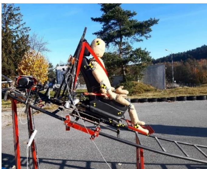
Fig. 13. KPSIT C50 dummy taking part in a frontal crash test using a passenger vehicle seat.
