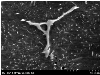
Fig. 13. Microstructure of transverse cross section, 7003S alloy sample, 4000x
