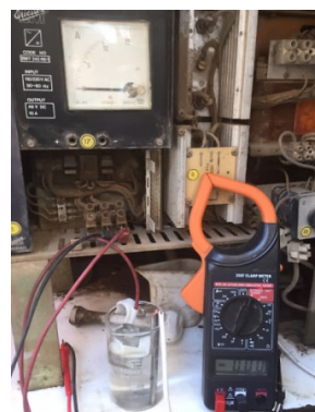
Fig. 6. The electrochemical cell and open circuit potential (OCP) test setup
