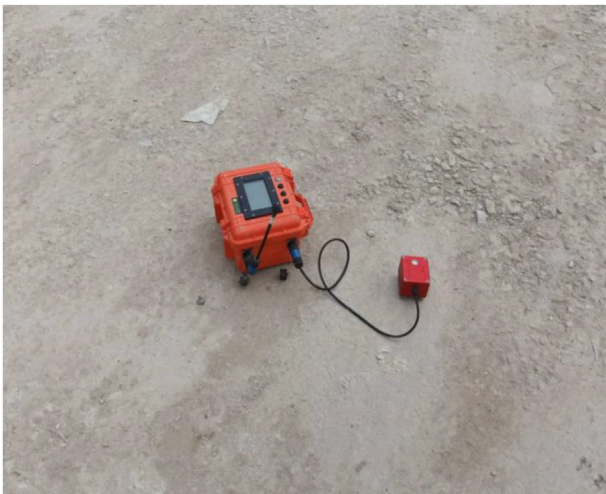
Fig. 3. Seismograph in position for noise and vibration measurement.
