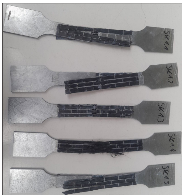
Fig. 8. Damaged first series samples – shear strength
