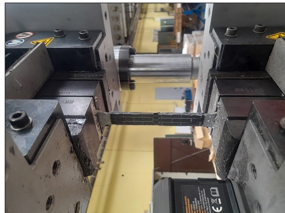
Fig. 4. Test stand - SK1 series specimen in the grips of a testing machine
