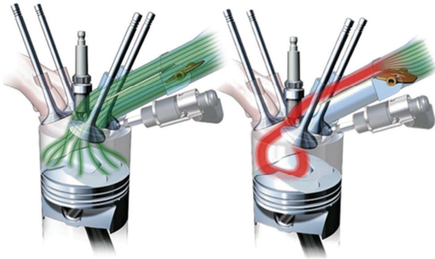
Fig. 2. The use of a turbulence generator in the form of a shutter in the inlet channel forcing a tumble motion of the gases (for example used in Audi 2.0 FSI engines) [15]
