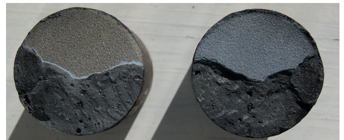
Fig. 11. Exemplary rupture of sample with coating sprayed with 97%Al 2 O 3 +3%TiO 2 powder
