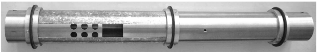
Fig. 2. An anemometr for measuring the distriubtion of the volumetric flow rate – a general view
