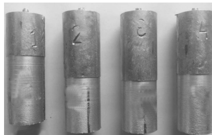
Fig. 1. The samples of the alloy AlSi7Mg0,3 before the exposition
