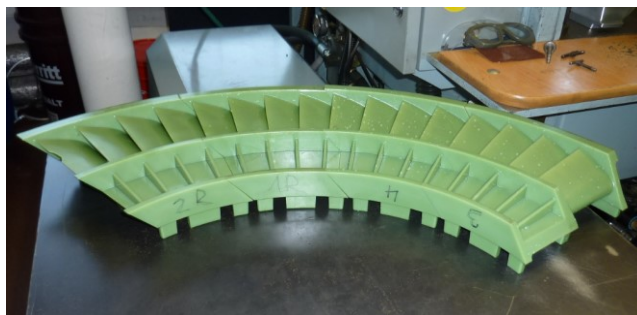
Fig. 2. Assembled wax patterns blade segment
