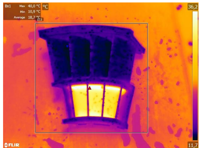
Fig. 12. Temperature on the B side after 10 minutes of cooling
