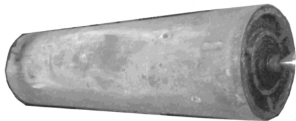
Fig. 2. Examined roller with clearly visible marks of wear of jacket's surface
