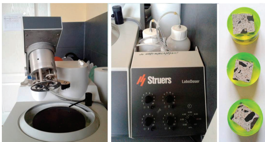
Fig. 3. (a) Polishing machine, (b) diamond suspension dozer, (c) of set polished samples
