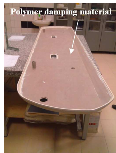
Fig. 10. Laminate bogie cover.
