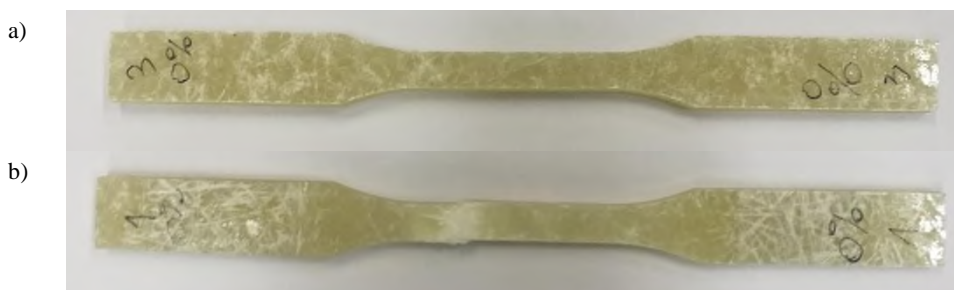
Fig. 2. View of specimens used in research: a) before, b) after the test
