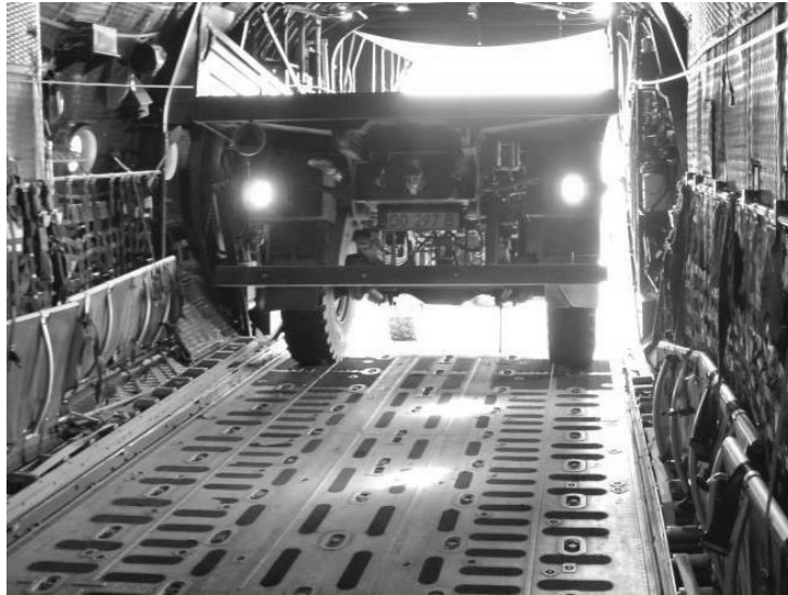
Fig. 2. View of fittings with the load capacity of 10000 ft in the C130E cargo bay
