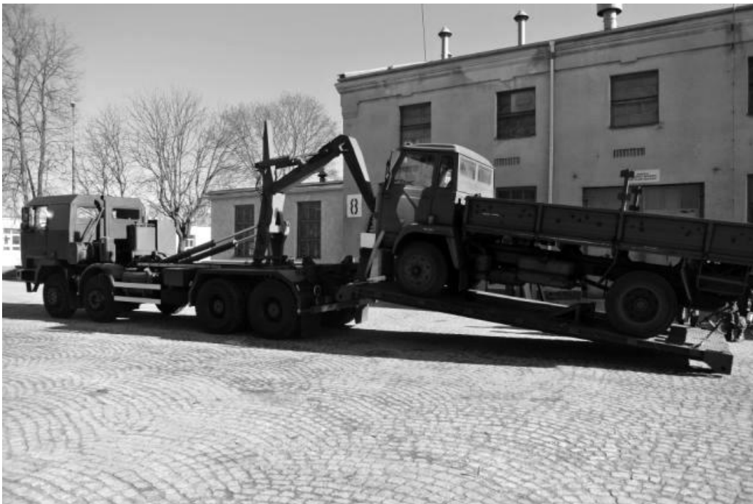
Fig. 11. The initial phase of loading a damaged car onto a high capacity vehicle using the Multilift Mk IV self-loading system
