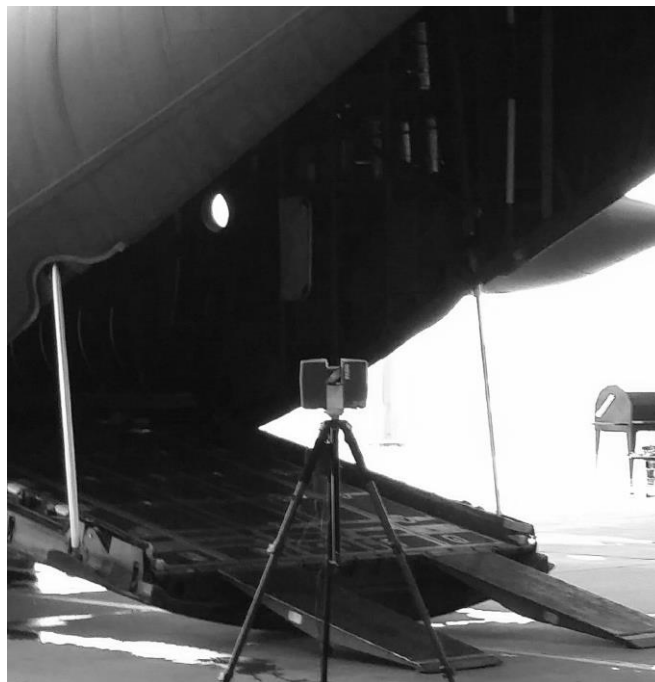
Fig. 13. Scanning of the cargo bay of the Hercules C-130 aircraft
