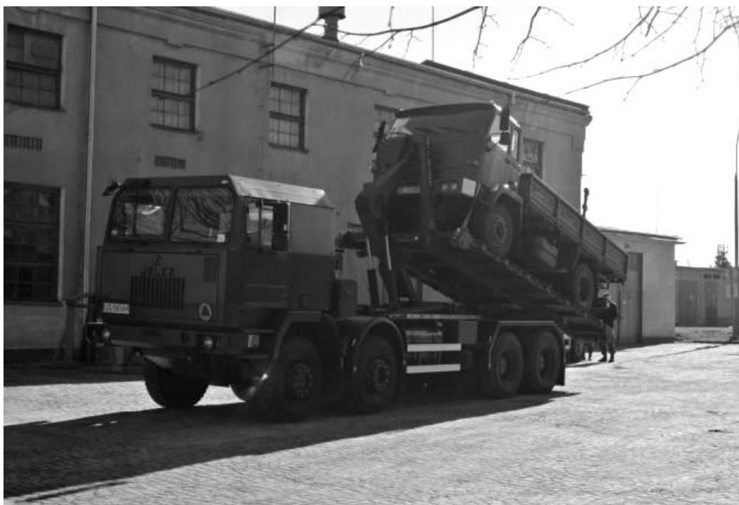
Fig. 12. The final stage of loading a car onto a high capacity vehicle using the Multilift Mk IV self-loading system
