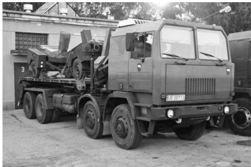
Fig. 10. Example of transportation of small vehicles on a high capacity vehicle - transport of 2 KPZ-170 type field kitchens
