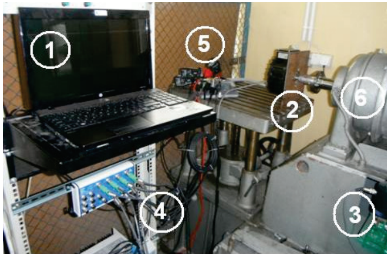
Fig. 6. Dyno test stand: 1 – acquisition equipment, 2 – electric engine, 3 – force sensor, 4 – acquisition hardware, 5 – current inverter, 6 – electric engine of the dyno stand
