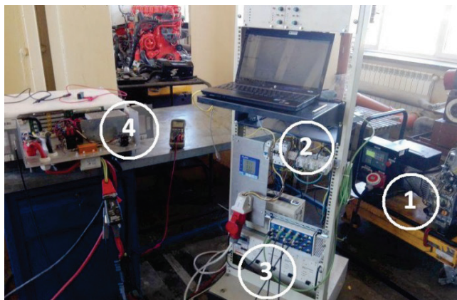
Fig. 1. Charging test stand: 1 – power generator 2 – current-voltage parameters acquisition system 3 – constant-current power station, 4 – battery
