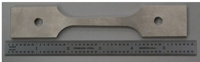
Fig. 2. Test specimen from Inconel 718 alloy [9]
