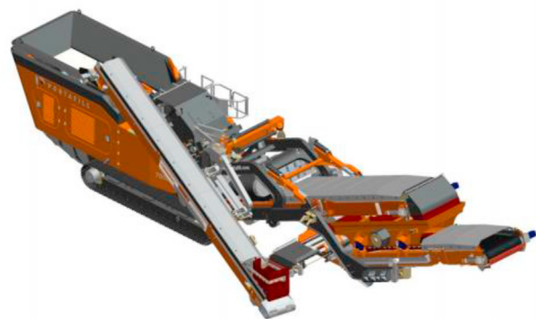
Fig. 4. Modern impact crusher with closed-loop. Source: [12].
