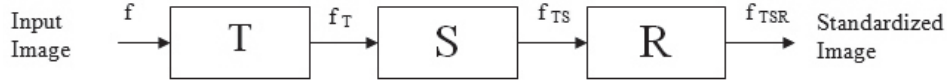
Fig. 3. Standardization of the input image which makes an object in processed images invariant to the translation (T block), scaling (S block) and rotation (R block)
