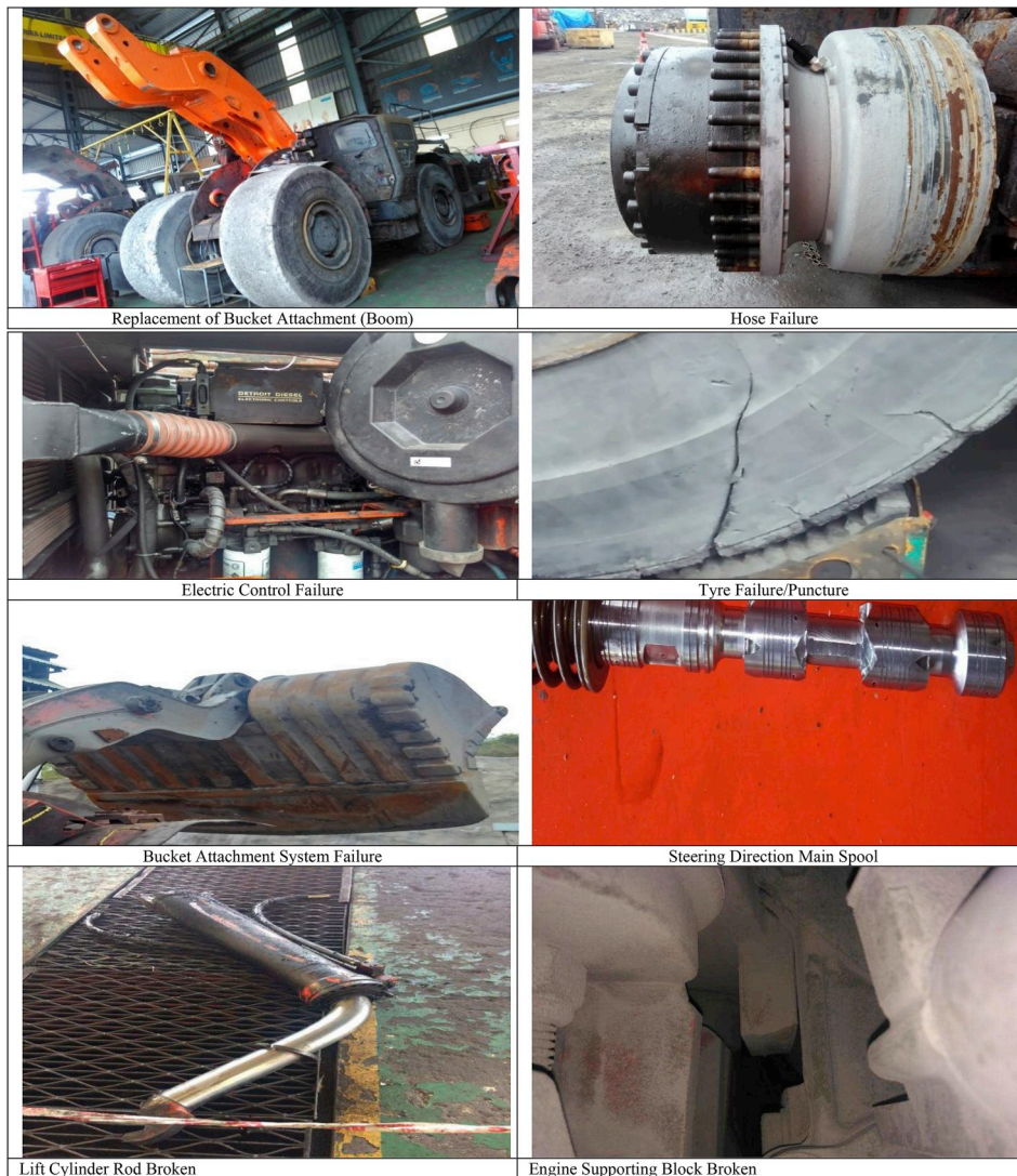
Fig. 4. Some potential failed parts of an LHD system.
