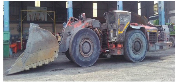
Fig. 3. A typical LHD system at a workshop for maintenance.
