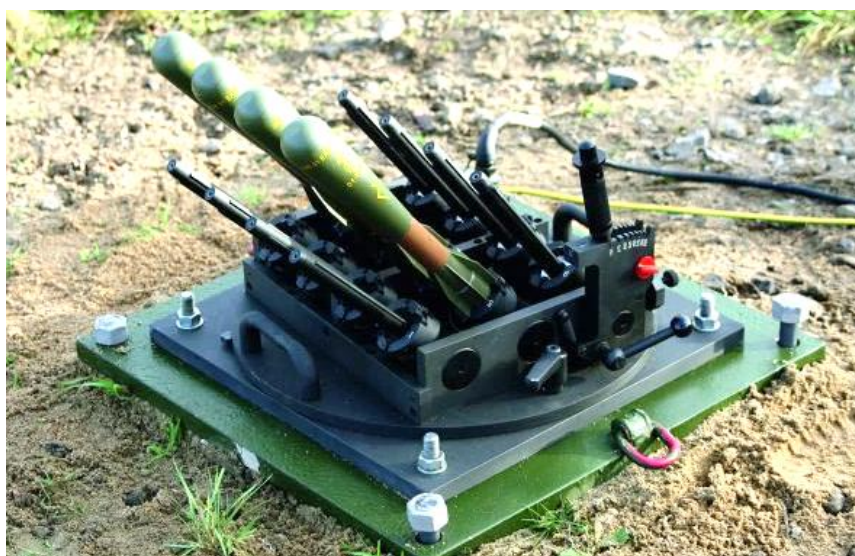
Rys. 5. Fly-K na platformie, załadowany 4 (max. 12) pociskami, zdalnie sterowany [7] Fig. 5. Fly-K on a platform, loaded with 4 (max. 12) projectiles, remotely controlled [7]
