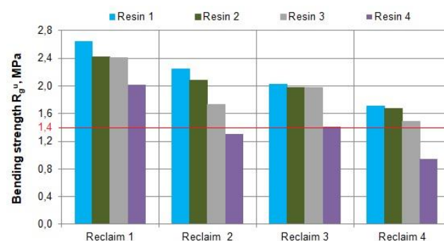
Fig. 2. The effect of the type of reclaim on the sand bending strength determined after 24 hours of hardening
