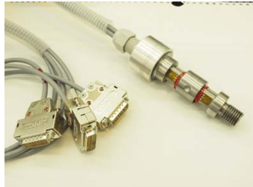
Fig. 3. Measuring bolt with installed strain gauge
