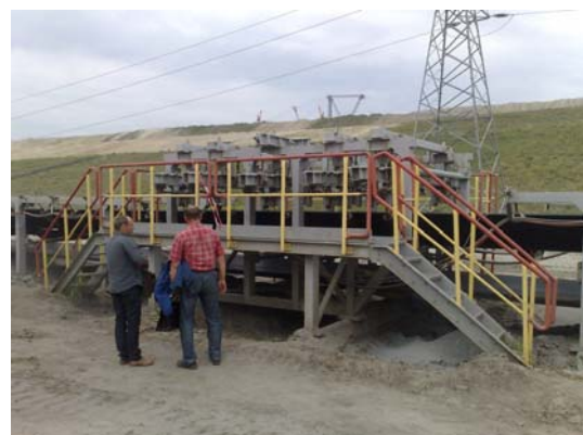
Fig. 4. Measuring unit assembled on construction of conveyor
