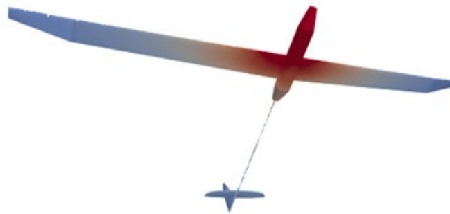
Figure 6. Results of sound pressure amplitude for both analysed sources (view from the bottom).
