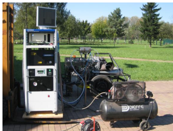
Fig. 5. Plan view of the measuring stand with GTD-350 engine
