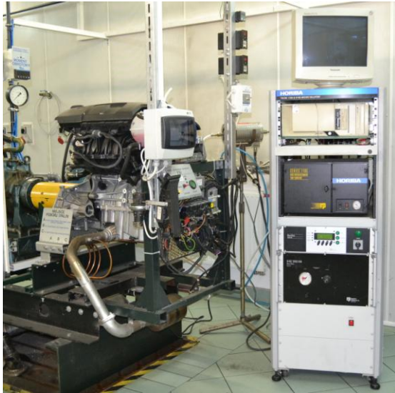
Fig. 1. Test stand with VW FSI 1,4 engine and Horiba TEOM 1105 analyser
