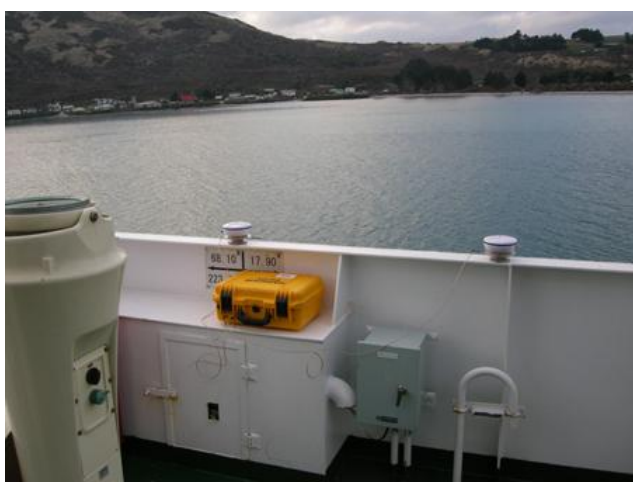
Fig. 2. An example of Portable Pilot Unit RTK type [source: www.navicomdynamics.com ]
