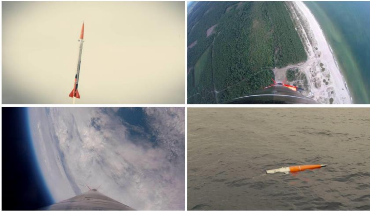
Figure 5. ILR-33 AMBER rocket flight test. Top-left – rocket’s ascent, note strap-on boosters still attached to the rocket. Top-right – the moment of strap-on boosters separation. Bottom-left – rocket in passive phase of the flight. Bottom-right – recoverable section of the rocket waiting for sea recovery. Own work of Ł-IoA.
