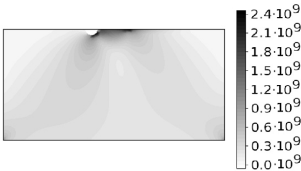
Fig. 4. Distribution of stresses in the studied structure given the presence of a concentrator, Pa
