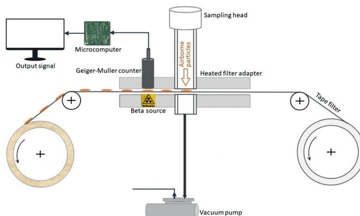
Fig. 1. The principle of MP101M analyser
