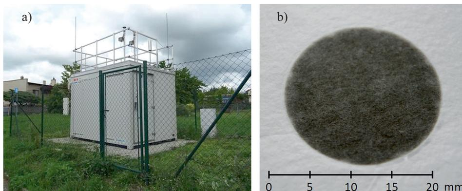
Fig. 2. a) Automatic imission monitoring station in Kutna Hora [24] and b) used fiberglass filter taken from MP101M particulate analyser after 24 hours of atmospheric air suction
