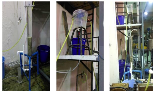
Fig. 6. Permeability test set up used in this investigation
