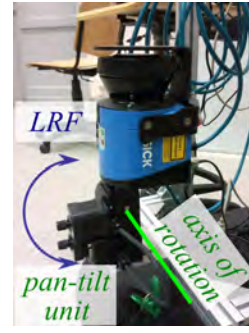
Fig. 7. The 2D LRF mounted on a pan-tilt unit used in our calibration
