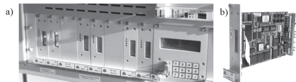
Fig. 7. The doubled modular processors and control level service keyboard in BUES 2000 signaling (a); View of modular processor single card (b) [own study]
