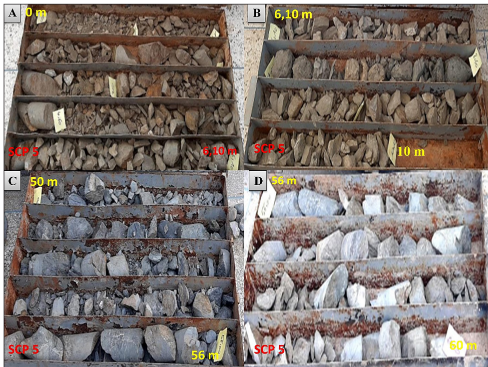
Figure 11. Core-drilling layers of the SCP 5 borehole
