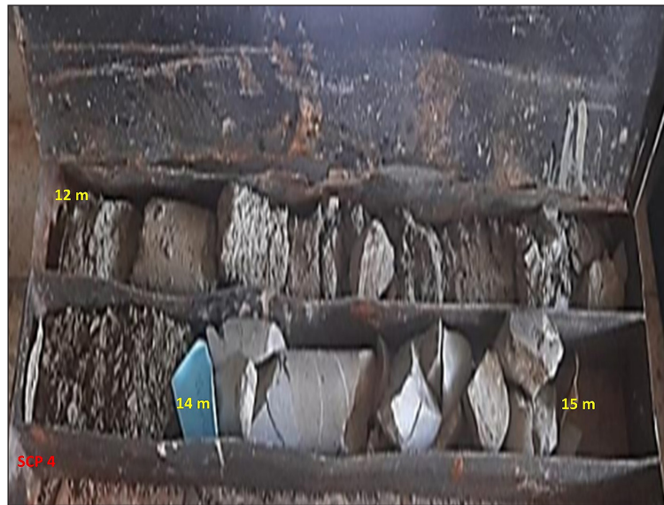
Figure 10. Core-drilling plates of SCP4 borehole between 12 and 15 m depth
