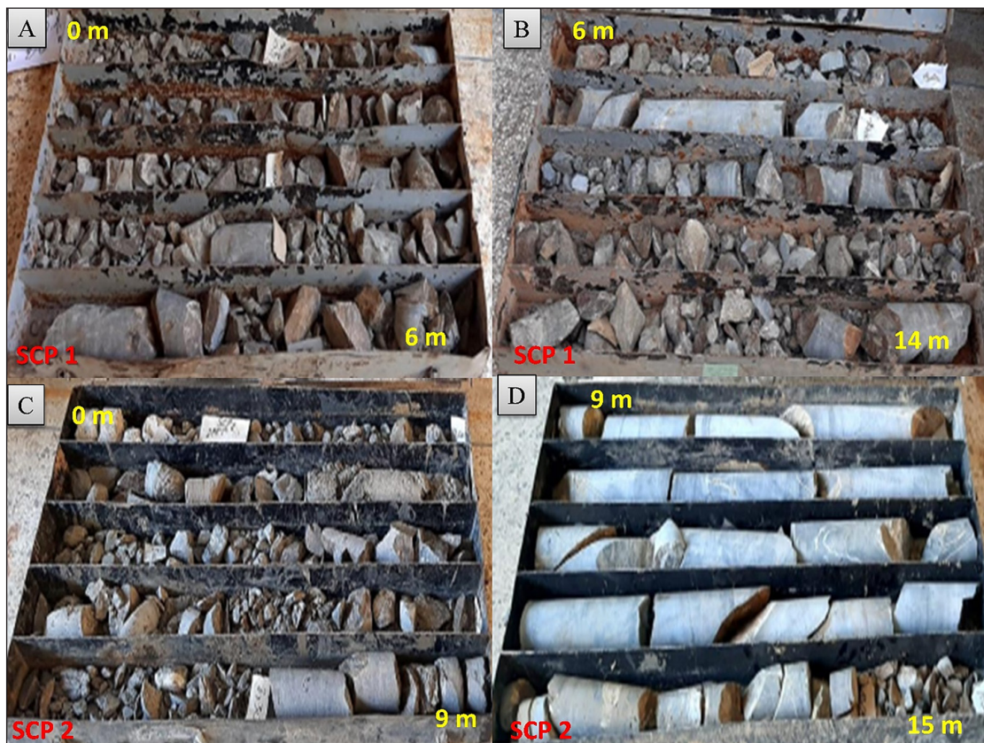
Figure 9. The first two core drilling plates SCP 1 & SCP 2: A SCP1 borehole from 0 to 6 m; B SCP1 borehole from 6 to 14 m; C SCP2 borehole from 0 to 9 m; D SCP2 borehole from 9 to 15 m
