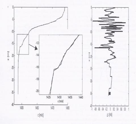
Fig.1. Profiles of sound velocity: as measured and following approximation
