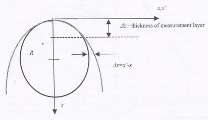
Fig. 3. A pictorial representation of how the circle equation describing the shape of the sound velocity profile in the measurement layer is replaced with a parabola equation
