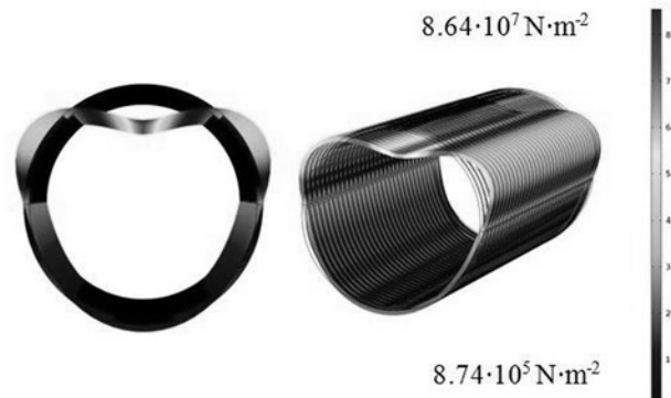
Fig. 7. Permanent deformation and distribution of the pressure stress due to radial force
