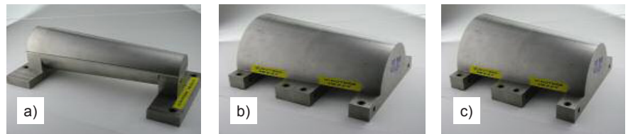
Figure 3. Types of anvils for testing acc. to HOSDB [4]; a) cylindrical, b) semicircular, c) convex.
