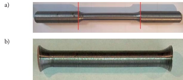
Fig. 7. Tested material sample: a) general view, b) selected (tested) sample segment
