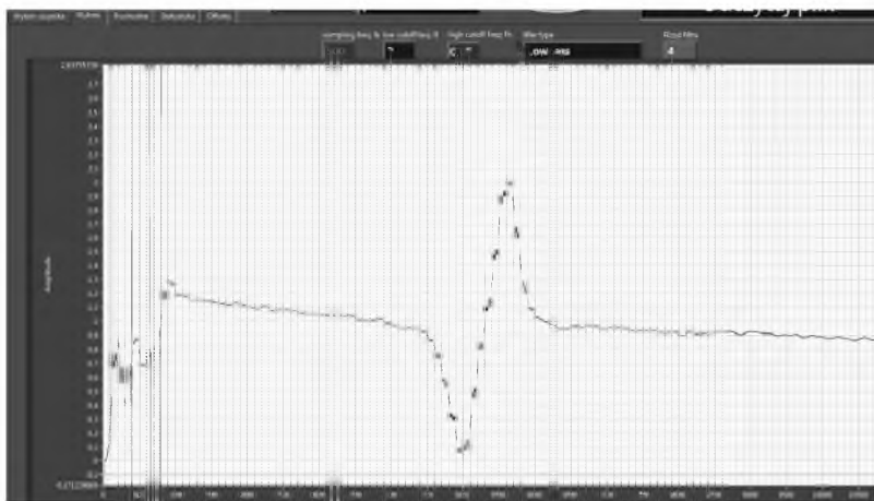
Fig. 11. Course of changes of the electric potential differences between the sensors No 9 and No 14
