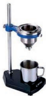
Rys. 1. Kubek Forda Fig. 1. Ford viscosity cup
