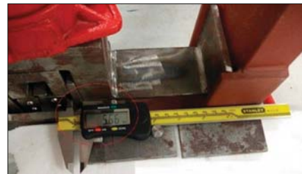
Fig. 3. Diagram of indirect measurement of embedded depth
