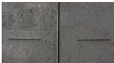
Fig. 5. Indentation of embedded blocks
