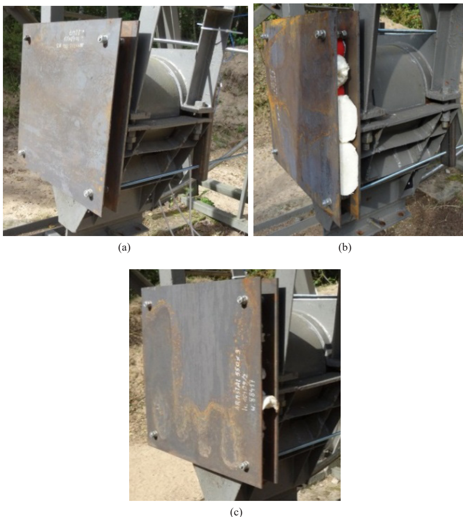
Figure 1. The tested material systems installed from the side of the mortar seat of the ballistic pendulum
