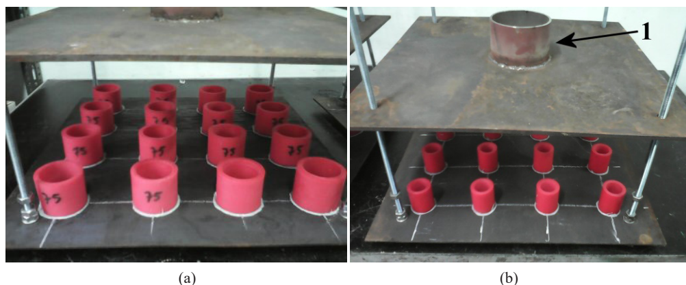
Figure 9. Assembling the tested material systems: 1 – aligning sleeve
