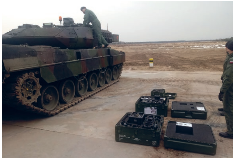
Fig. 7. Installation of the AGDUS simulator on LEO2A5 by AWL cadets Source: Own study.
