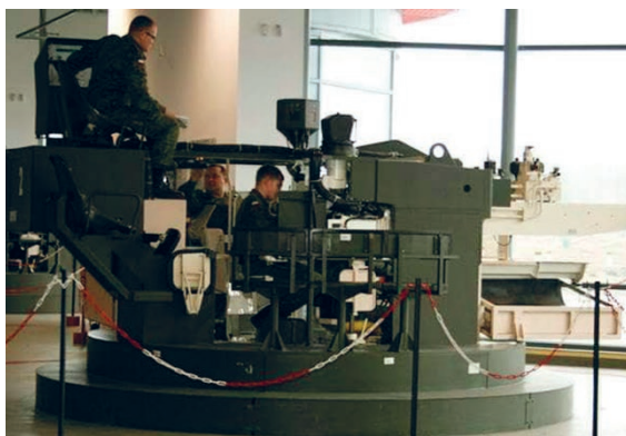
Fig. 3. One of the three AAT trainers used in the Leopard Training Center at the 10BK Panc in Świętoszów Source: [8].
