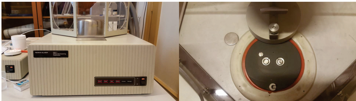
Fig. 1. Perkin Elmer Differential Scanning Calorimeter DSC-7.....Fig. 2. DSC apparatus, inside of measuring cell
