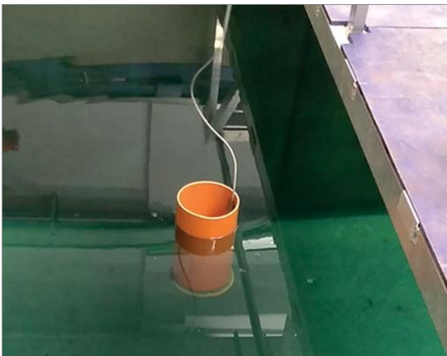
Fig. 6. Model tests of a damping ring cylinder
