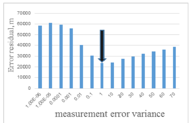
Figure 7. Cumulative error difference between true and smoothed positions against measurement error variance.
