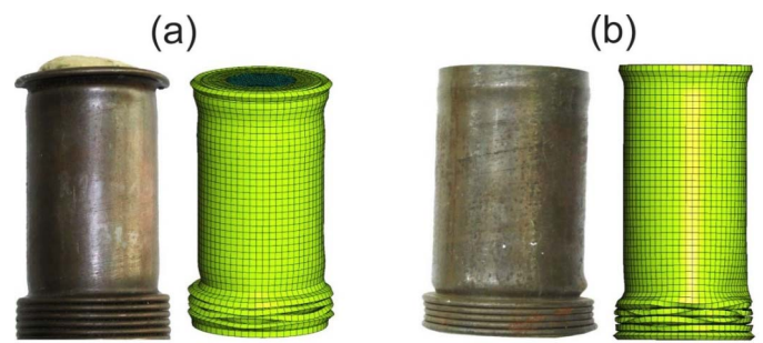
Fig. 13. Comparison of post-crash geometry of 160 kg/m 3 foam filled tubes: a) single-wall, b) double-wall
