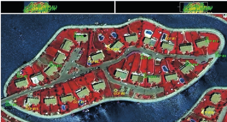
Fig. 3. Distribution of 10 well distributed control points (yellow color) and 10 well distributed check points ICPs (green color)
