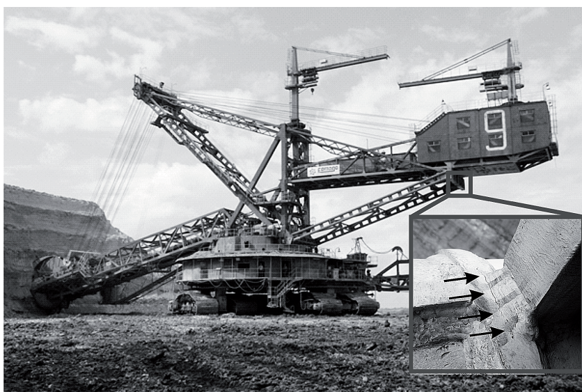
Fig. 1. Developing fracture crack
