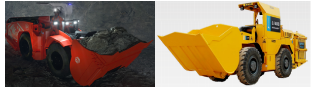
Fig. 3 Selected models of BEV LHD loaders (Artisan A4 model, Aramine L140B model)
